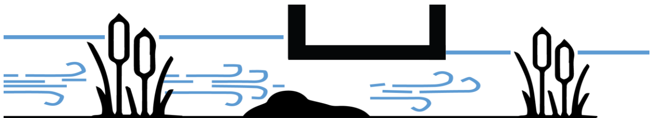
Figure 79 Friction and flow obstruction in and around culverts (Jos Muller, August 2016)
