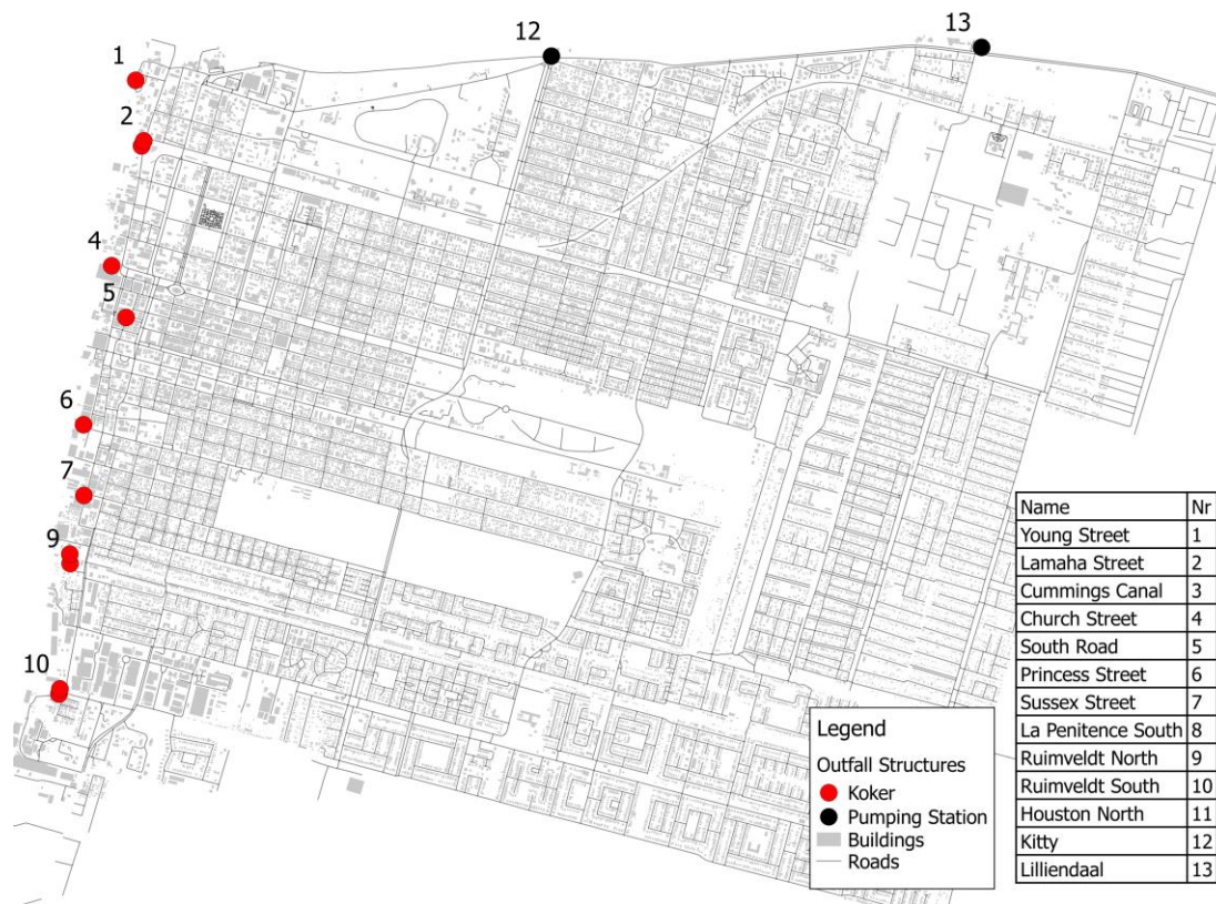
Figure 41 Overview of outfall structures in Georgetown, Guyana (Openstreetmap, 2016)
