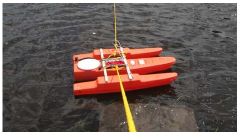
ADCP (above), example river velocity profile (below) and the sound-emitting ADCP transducers (top right)
